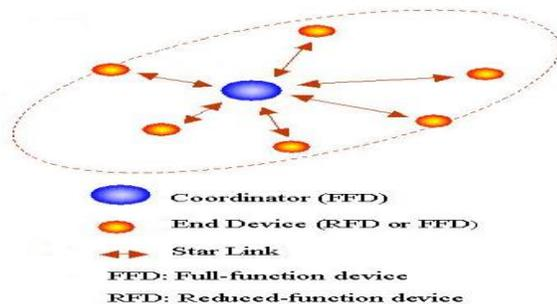
Wireless pan(WPAN) focuses on low-cost, low-speed ubiquitous communication between devices. WPAN has a range of 10-100 meter communications area which Transfers at a rate up to 250 Kbit/s.It is also used for secure communications and can be used in any topology that Uses Offset Quadrature Phase Shift Keying (OQPSK) modulation. WPAN uses 2400-2483.5Mhz frequency band
